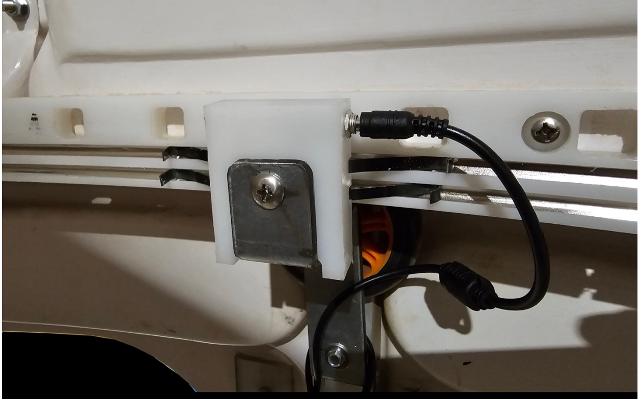
9- Connect the limit switch and power plugs to the shutter motor unit.
